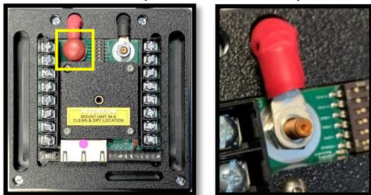
4. Feed the LVBP ring terminal up through slot & place the LVBP ring terminal on the stud of the positive terminal. Tighten 3/8" nut **(DO NOT OVER TIGHTEN)**. Place red cap back onto positive terminal.
